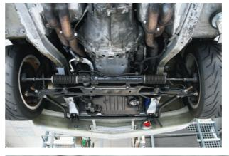
"We welded in a new, larger transmission tunnel to take the modern six-speed gearbox, and the suspension turrets were all replaced with new, reinforced ones"
