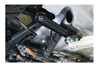
Michael began the mechanical installation. The suspension is KW's Phase 3 coil-over system with motorsport grade rose-joints used on all the suspension arms and top mounts.
